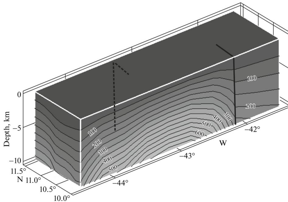
**Fig. 3.** Three-dimensional block diagram of temperature distribution ( $^{\circ}\text{C}$ ) along the Vema transform fault. Thick lines show the position of fragments of the Mid-Atlantic Ridge (solid line, to the south of the fault; dotted line, to the north of the fault).
