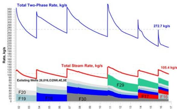
**Figure 5: Forecasting modeling (scenario EX3A) of total two-phase, total steam production of wells (existing wells 016, 26, E4, 029W, E5 and additional F-wells) at Dachny site, Mutnovsky geothermal field**
