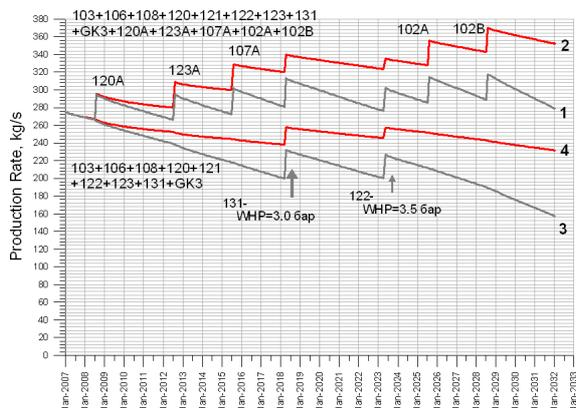
**Figure 2: Predicted total two-phase production rate for Pauhetsky: 1 - Wells 103, 106, 108, 120, 121, 122, 123, 131, GK3, 120A, 123A, 107A, 102A, and 102B for the 2007–2032 period (Kiryukhin et al, 2008); 2 – the same, as 1, but with disabled infiltration areas; 3 - steam rates using only wells existing on December 2006 (Kiryukhin et al, 2008); 4 - the same, as 1, but with disabled infiltration areas**
