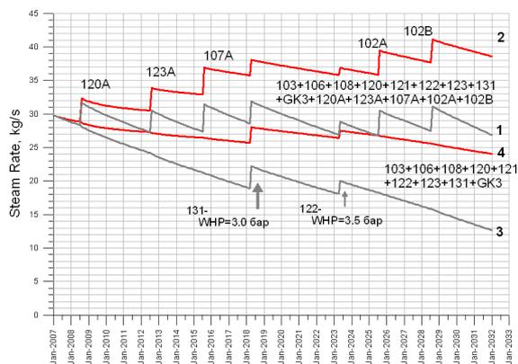
**Figure 3: Predicted total steam production rate for Pauhetsky: 1 - Wells 103, 106, 108, 120, 121, 122, 123, 131, GK3, 120A, 123A, 107A, 102A, and 102B for the 2007–2032 period (Kiryukhin et al, 2008); 2 – the same, as 1, but with disabled infiltration areas; 3 - steam rates using only wells existing on December 2006 (Kiryukhin et al, 2008); 4 - the same, as 1, but with disabled infiltration areas. The steam rate is calculated at the separation pressures of corresponding wells**
